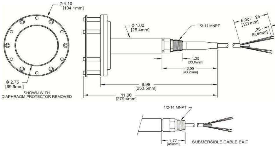
Molded Cable Seal Configuration for Polyurethane Cable
