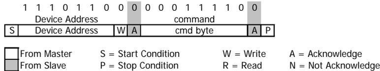
Figure 5: I<sup>2</sup>C Reset Command
